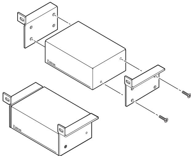
**Figure 4 — Attaching the back of the rack kit**
