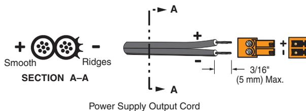
**Figure 3.** Wiring the Power Connector
