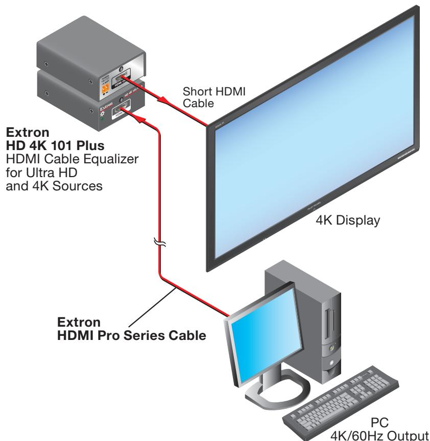
**Figure 1. HD 4K 101 Plus Application Diagram**
