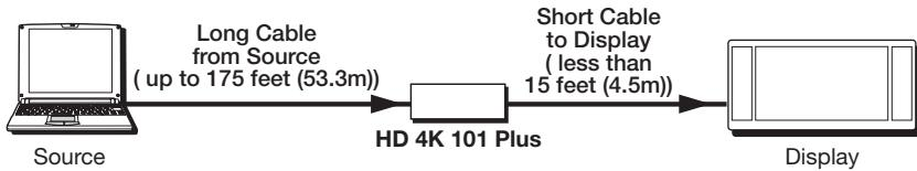
**Figure 5. Optimum Cable Lengths for the HD 4K 101 Plus**
