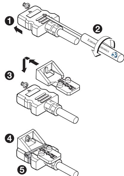
4. Loosely place the included tie wrap around the HDMI connector and the LockIt lacing bracket as shown.
