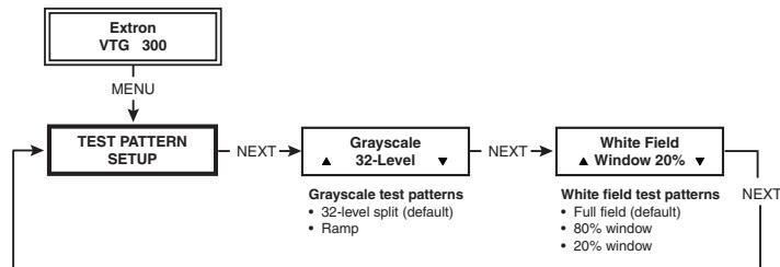
**Figure 2-3 — Test Pattern Setup menu**
