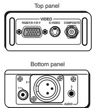
The video connectors located on the top panel will accommodate RGB, component, S-video, and composite video output.
