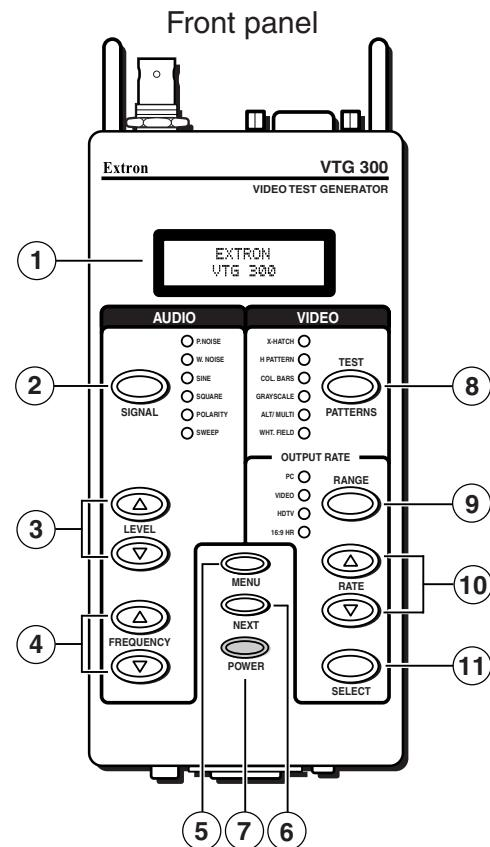
④ **Audio frequency adjustment (Frequency)** — When the audio signal type is either a sine or square wave (see ② above), the audio frequency can be adjusted from 20 Hz to 20 kHz (sine) or 20 Hz to 5 kHz (square). Press the ▲ button to increase the frequency and the ▼ button to decrease the frequency. The adjustment is in 1/3 octave steps. See *Setting the Audio Frequency* in this chapter.
