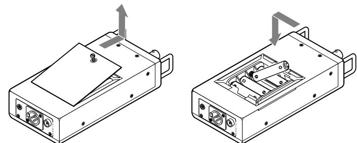
Figure 2-14—Battery installation
