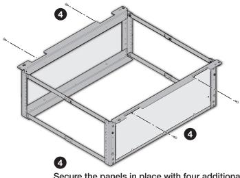
Secure the panels in place with four additional mounting screws at the top.
