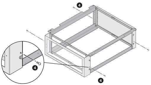
Lock each panel in place with two of the included #10-32 x 0.25 inch Phillips truss-head screws.
