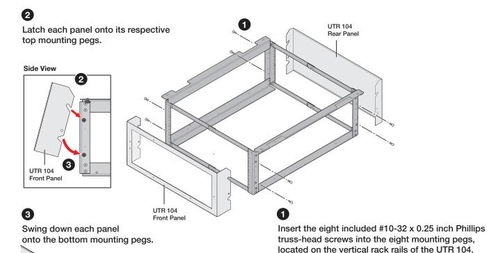
Figure 1. Installing the UTR 104 FRP
