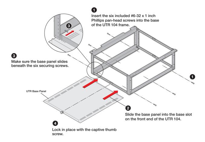
Figure 1. Installing the UTR BP
