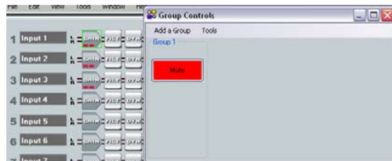
Figure 5-10 — Sample mute group master and muted inputs
