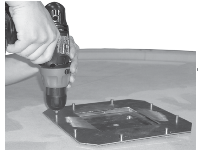
Figure 2-2 — Using the drilling template
