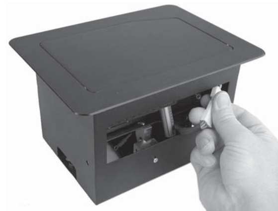
Figure 1-4 — Disconnecting the interior AC cable
