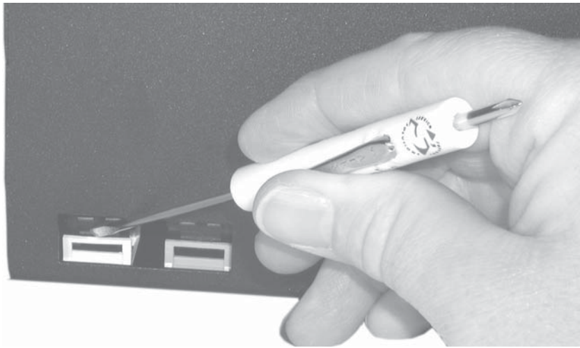
Figure 1-6 — Releasing the bezel plug-in detent
