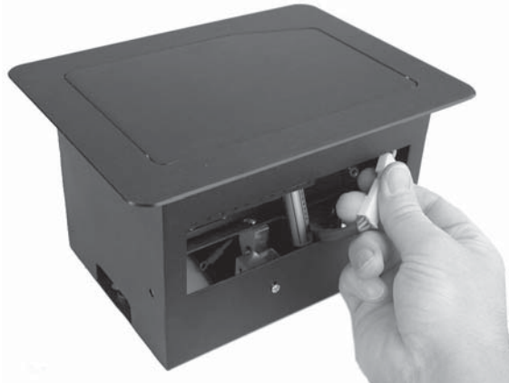
Figure 1-4 — Disconnecting the interior AC cable
