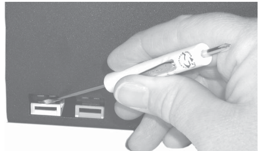
Figure 1-6 — Releasing the bezel plug-in detent
