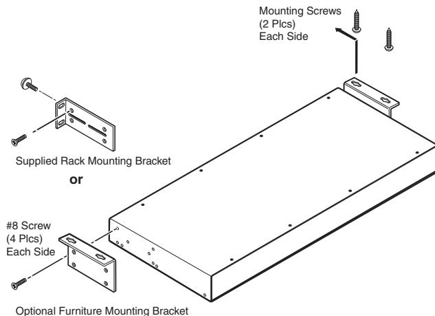
**Figure 2-1 — Mounting the DA**
