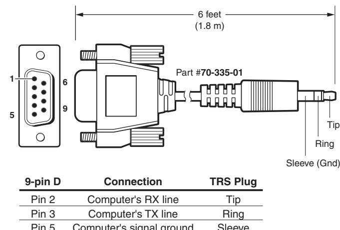
**Figure 2-9 — Optional 9-pin TRS RS-232 cable**
