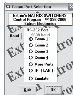
2. Choose the comm (serial) port that is connected to the switcher or **IP [ LAN ]**.
