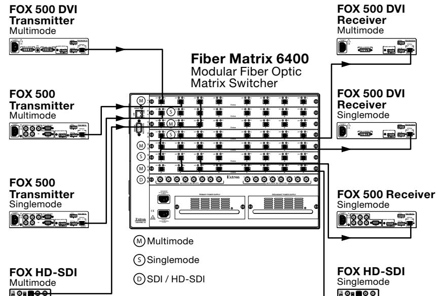
**Figure 1-1 — Typical Fiber Matrix 6400 application**
