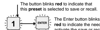
The Enter button blinks red to indicate the need to activate the save or recall.
