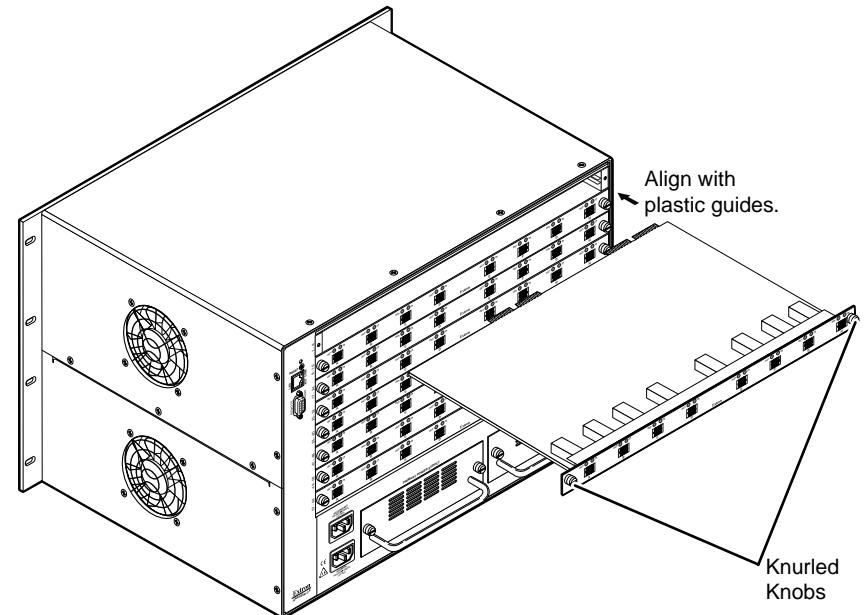
5. Place the removed board on an anti-static surface or in an anti-static container.
