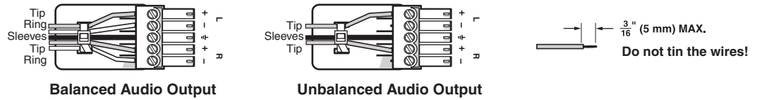
Figure 4. Audio Output Connector Wiring
