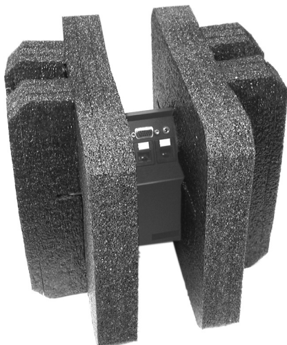
Figure 35. HSA Unit Suspended in the Foam
