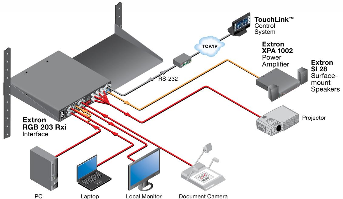
**Figure 1. Typical Application for the RGB 203 Rxi**
