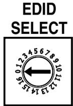
**NOTE:** Configuring the rotary and DIP switches allows a user to select a pre-programmed EDID setting based on the native rate of a display (for example, 1024x768) and a desired frequency (50 or 60 Hz), but does not necessarily force a video source to output that rate.
