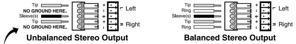
**CAUTION:** For unbalanced audio, connect the sleeves to the center contact ground. **DO NOT** connect the sleeves to the negative (-) contacts.
