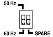
The second DIP switch is not used by this device.
