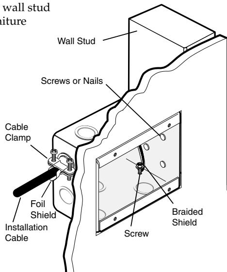
To attach the wall box to wood, use four #8 to #10 wood or sheet metal screws. A minimum of 1/2" (1.3 cm) of screw threads must penetrate the wood. If the wood is a 2 x 4, such as a wall stud, 10-penny or larger nails can be used.
