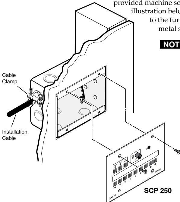
**NOTE** *If you are not installing the SCP into a grounded metal wall box, make sure that the faceplate is grounded to an earth ground.*
