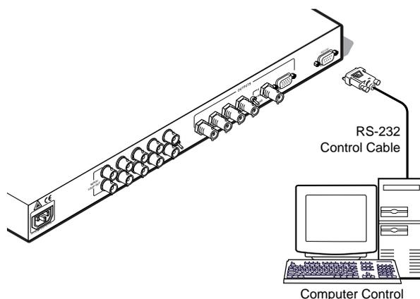
**Figure 9 — DDS 100 scaler RS-232 to host connection**
