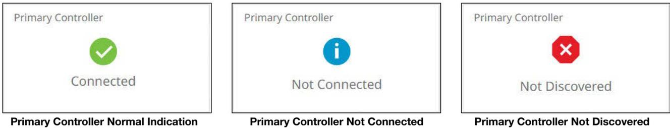
**Figure 33.** Primary Controller Pane Indications
