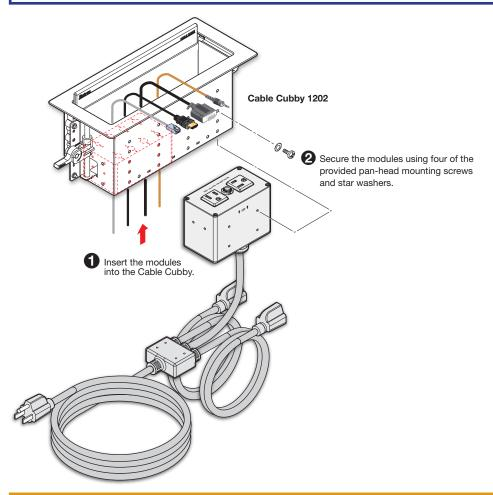
**WARNING:** Risk of Electric Shock. To ensure proper electrical grounding, use the provided #6-32 mounting screws with the star washers.
