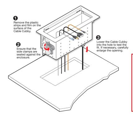
**CAUTION:** The flanged edges of the top of the surface enclosure are sharp. These edges are also soft and may be easily nicked or bent. Exercise caution when handling the enclosure to prevent personal injury or damage to the enclosure.
