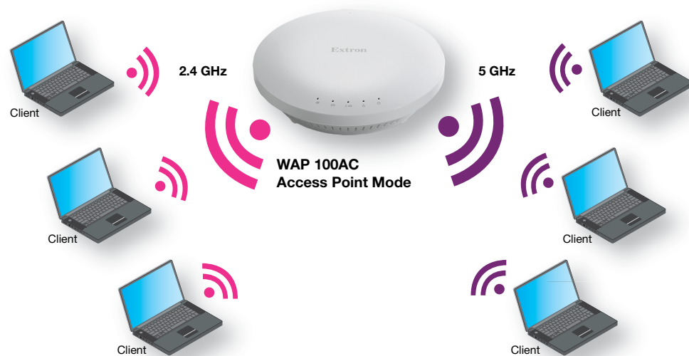
Figure 32. Access Point Mode
