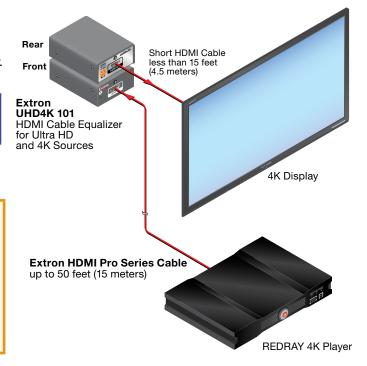
**NOTE:** If all the devices are correctly cabled and powered on and you do not see an image on the display device, you may need to buffer the DDC signal (see the *UHD4K 101 User Guide*).
