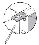
**ATTENTION:** Do not drill through the table or furniture. If the table is too thin or of a different material for the supplied screws, use an appropriate type and length.
