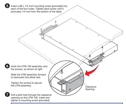
NOTE: If necessary for easier access, mark the location of the clearance opening, then remove the UTM system to drill the hole.
