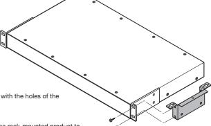
Align the holes of the UTM 100 with the holes of the rack ear, as shown at right.
