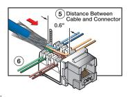
Use the 110-style punchdown tool to push down each wire into the IDC slot. Push the punchdown tool until the wire is firmly secured at the bottom of the slot.
