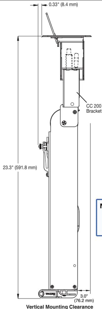
**NOTE:** To prevent objects from impeding cable retraction, ensure at least 3 inches of clearance from the exposed cable side of the enclosure.
