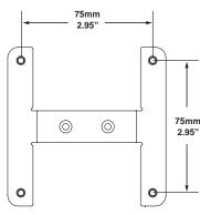
The Extron® VM 700T is an adapter that provides a VESA-mounting option for the TLP 700TV TouchLink<sup>™</sup> panel.
