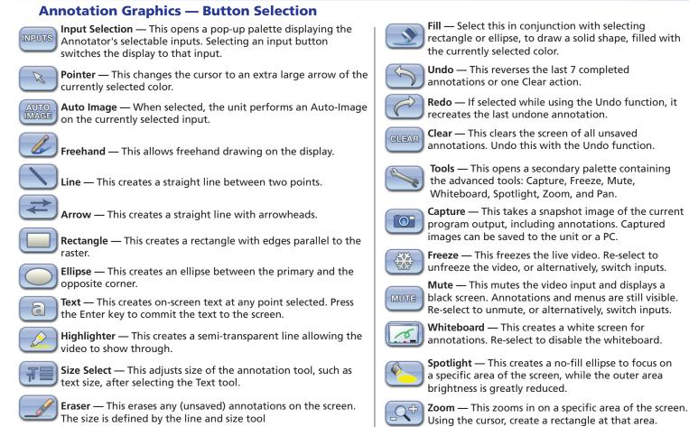
**Color** — This allows up to 16 colors to be selected for any drawing function (fill or outline), text, or pointer.
