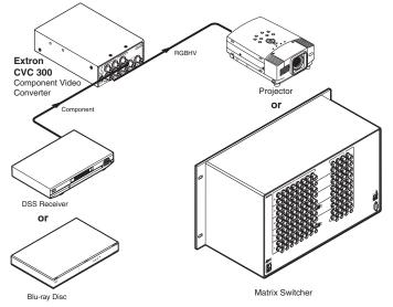
The component video input formats include SMPTE, HDTV and Betacam component video. The RGsB video input can be computer video or NTSC/PAL video.
