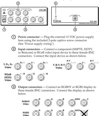
Power LED — Green when power is applied and an active video input is detected. Amber if power is available but no input signal is present.
