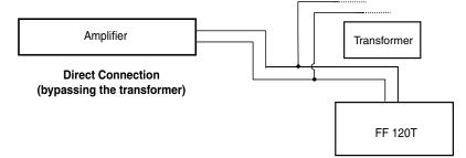
b. Connect the red positive (+) wire to the + speaker terminal and connect the black negative (-) wire to the - speaker terminal, depending on whether one or two speakers are being connected, as shown below.
