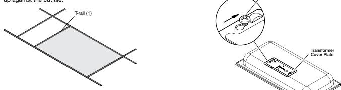
4. **Transformer cover plate** — Loosen, but do not remove, the two screws on the top of the transformer cover plate, as shown at right. Next, slide and remove the transformer cover plate, which is installed with the transformer side down.
