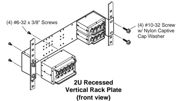
Note: Fill unused holes in rack plates with plastic plugs (included)
