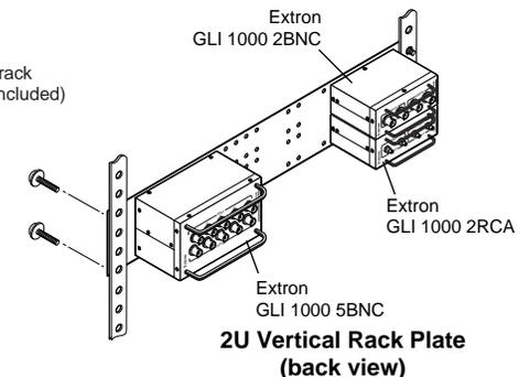
1. Use four #10-32 rack-mounting screws and washers to mount the plate to the rack. See the illustration above.
