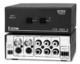
The Extron YCS SW2 A is a two input, dual output video and audio switcher with built in video transcoding. It simultaneously decodes composite video signals into S-video signals, and encodes S-video signals into composite video signals. The YCS SW2 A is ideal for simplifying signal routing to video projectors and other display devices in A/V systems designed for classrooms, conference rooms, and video conferencing.
