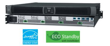
The ENERGY STAR qualified **XPA U 4004 FX** uniquely features ECO Standby, that works with InstaWake+ to provide exceptional energy savings. ECO Standby automatically maximizes the time the amplifier operates in its lowest possible power state, while InstaWake+ gives the amplifier the ability to return to full power from standby in under 5 milliseconds.
