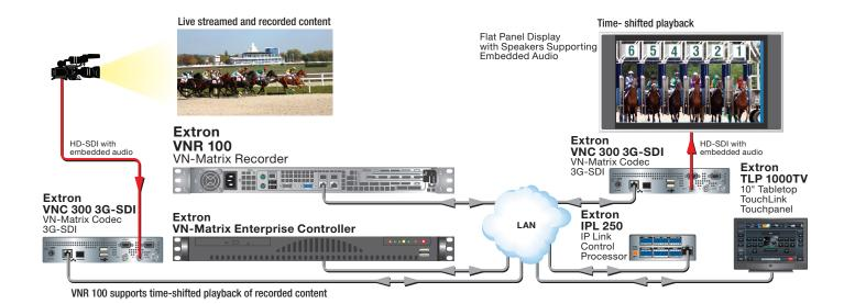
recording systems can be programmed and managed from a single point using VNM Enterprise Controller.
