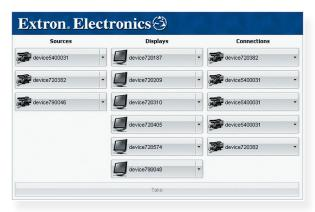
VN-Matrix Enterprise Controller Switcher utility connects encoder inputs to decoder
