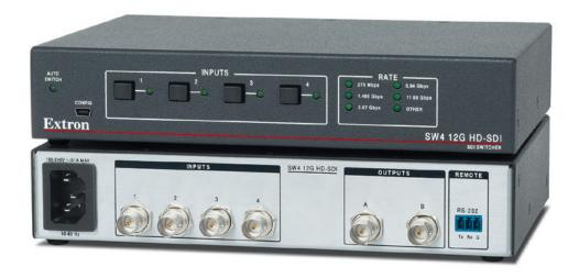
The Extron SW4 12G HD-SDI is a four-input, two-output 12G-SDI switcher that supports video resolutions up to 4K/60 and data rates up to 11.88 Gbps. It switches multi-rate SDI video, embedded audio, and other ancillary data between four source devices and delivers simultaneous output signals to a pair of SDI displays or sink devices. The SW4 12G HD-SDI switcher is ideal for integration into a variety of applications and environments.
