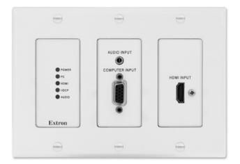
The Extron FOX T UWP 302 Fiber Optic Transmitter is a two input decoratorstyle switcher for long haul transmission of HDCP-compliant HDMI, RGBHV, or HD component video and stereo audio over fiber optic cabling. With support for digital and analog video signals in a wall-mountable design, the FOX T UWP 302 is ideal for signal switching and long haul transmission in a wide range of applications.
