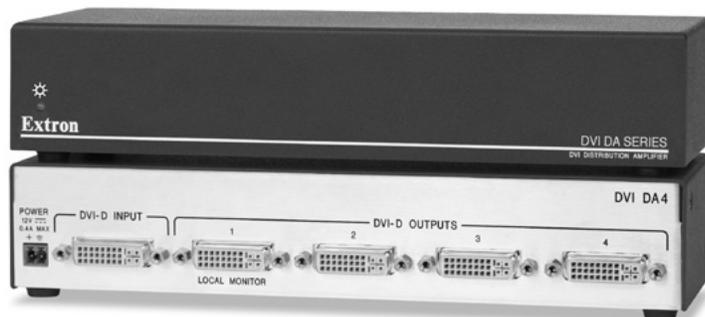
The Extron DVI DA distribution amplifiers with two or four outputs accept a single link DVI input signal and output multiple identical signals to attached devices. These distribution amplifiers provide automatic input cable equalization to ensure optimal image quality on all outputs. The DVI DA distribution amplifiers are ideal for use in all applications that require reliable distribution of high resolution DVI digital video signals.
