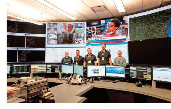
For control, each operator workstation includes a PC loaded with Extron EMS Express Mobile Software that facilitates content selection and display in customized windows arranged across the videowall.
