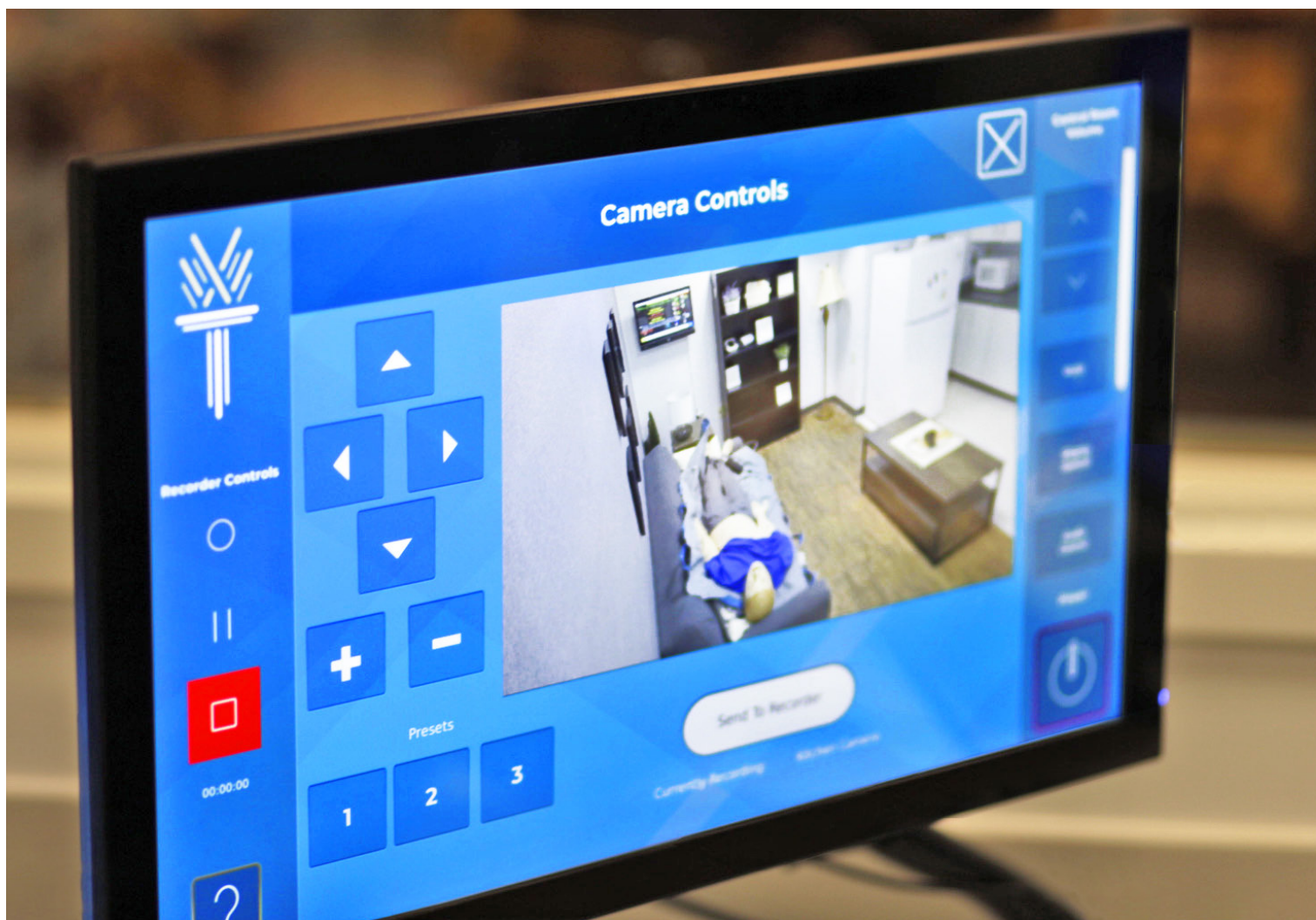
A 24" touchscreen controls all AV functions including PTZ camera positioning. The touchscreen connects to the Extron control processor via a TLI Pro 101 TouchLink interface.
