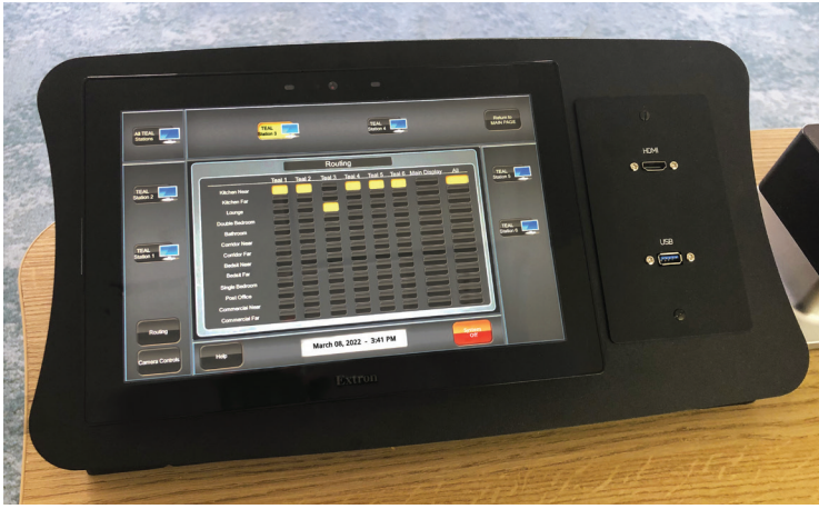
The instructor is able to control all AV signal routing using a single screen on the Extron TLP Pro 1025M 10" TouchLink® Pro Touchpanel mounted to the lectern.
