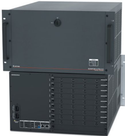
The Quantum Ultra 610 processor is configured with a mix of IN4HDMI input and OUT4HDMI output cards. It receives AV source signals over HDMI from an Extron XTP II CrossPoint 6400 matrix switcher.
