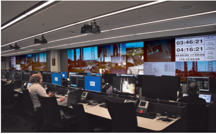
DOSC's two videowalls driven by Quantum Ultra processing support approximately 100 engineers with video and telemetry capabilities for day-of-launch activities.
