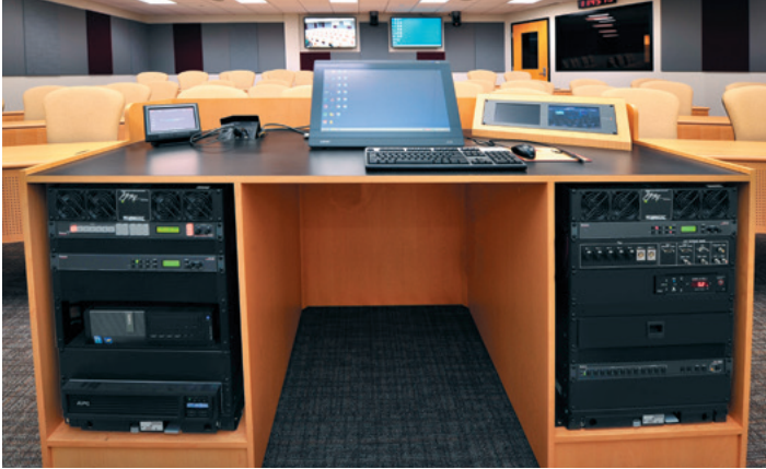
In the classroom, the Annotator provides instructors with the ability to make notations to computer-video presentations and over live video from campus cable or the DVD/VCR player.
