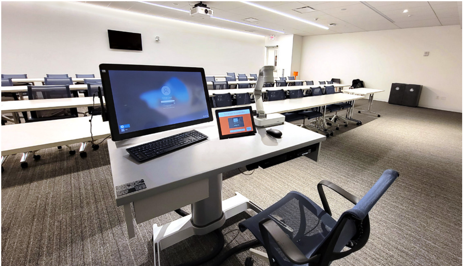
The standard classroom presentation workstation is a Steelcase AirTouch height-adjustable table outfitted with a micro-PC, an annotation touch screen, a Blu-ray® player, a document camera, AV connectivity with power, and an Extron TLP Pro 1025T 10" Tabletop TouchLink Pro Touchpanel for system control.
