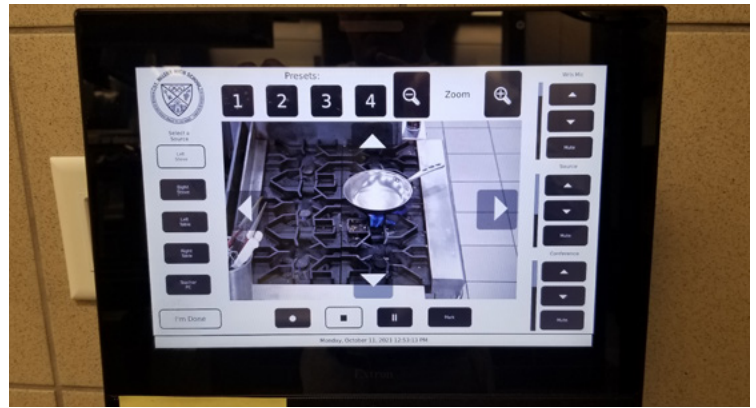
The chef uses the Extron TLP Pro 1225TG 12" Tabletop TouchLink® Pro Touchpanel installed next to his computer to control the AV system, including selecting among the camera presets.
