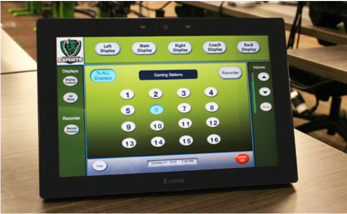
Coach Gaul controls the XTP system using the TLP Pro 1025T 10" Tabletop TouchLink® Pro Touchpanel at his workstation.
