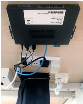
The HC 404 switching transmitter mounted beneath the conference table (left) extends user audio, video, and control to the ceiling-mounted projector located up to 230 feet (70 meters) away over CATx cable via an HC 404 scaling receiver mounted above the ceiling (right). Also shown on the left is a cable retractor installed beneath the table.
