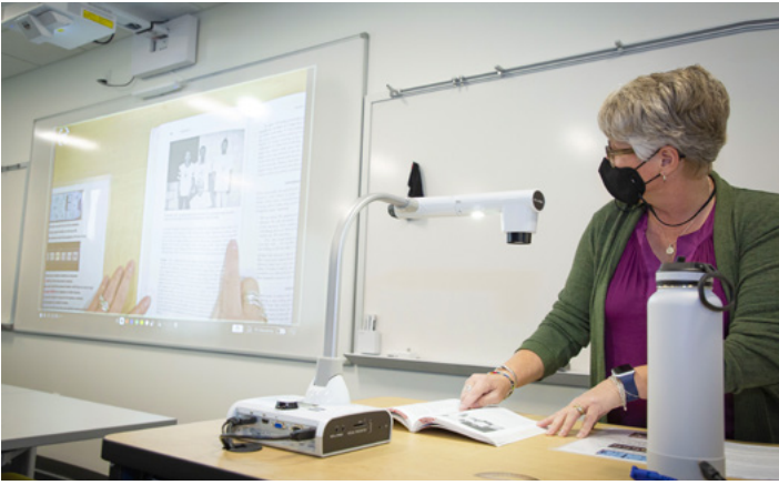
Classroom AV system in a typical setting. Here, the instructor is projecting an image from the document camera.
