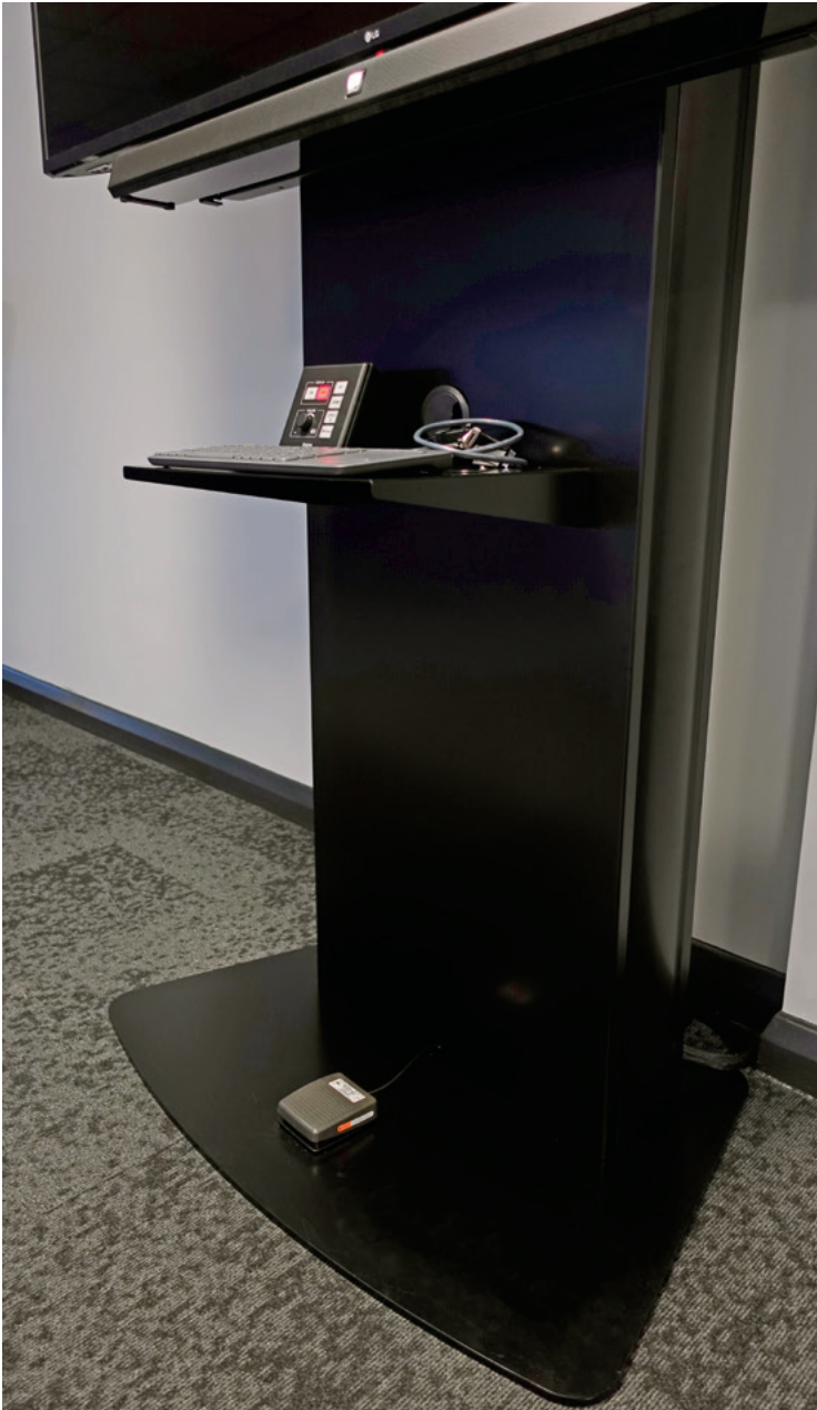
Primary Stands include a foot switch that provides no-touch control of main power and AV source selection.
