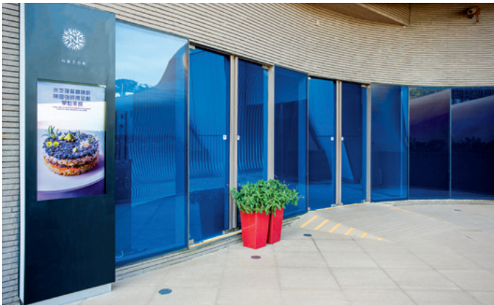
At the restaurant's entrance, a 46" LED outdoor signage display entices diners with previews of the chef's creations awaiting inside. The display receives HDMI video from the matrix switcher via DTP twisted pair cables that carry the signal over the extended distance from the AV equipment rack located inside the building to this exterior location.
