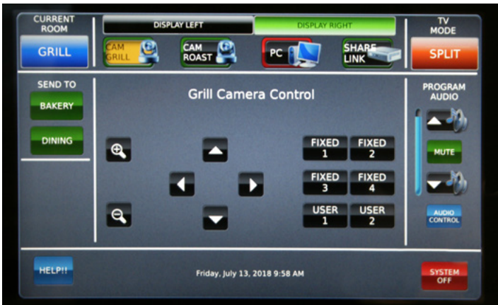
The full-motion video touchscreen on the TouchLink Pro touchpanel allows the instructor to easily preview and select the best camera angle when preparing to demonstrate a cooking technique.
